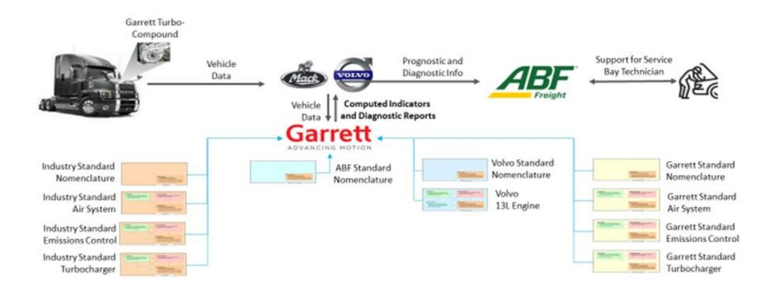
The Program Uses HRCS Provided Templates and Datasheets to Compute JA6268 Compatible Indicators and Diagnostic Reports
